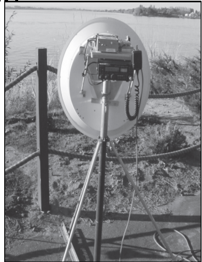
Figure 4.14 — N7CFO's dish antenna operates on 10 GHz and is portable enough to be taken on contest outings.
