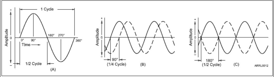
Position within a cycle is called *phase*. Phase is used to compare how sine wave signals are aligned in time. Measured in degrees.
